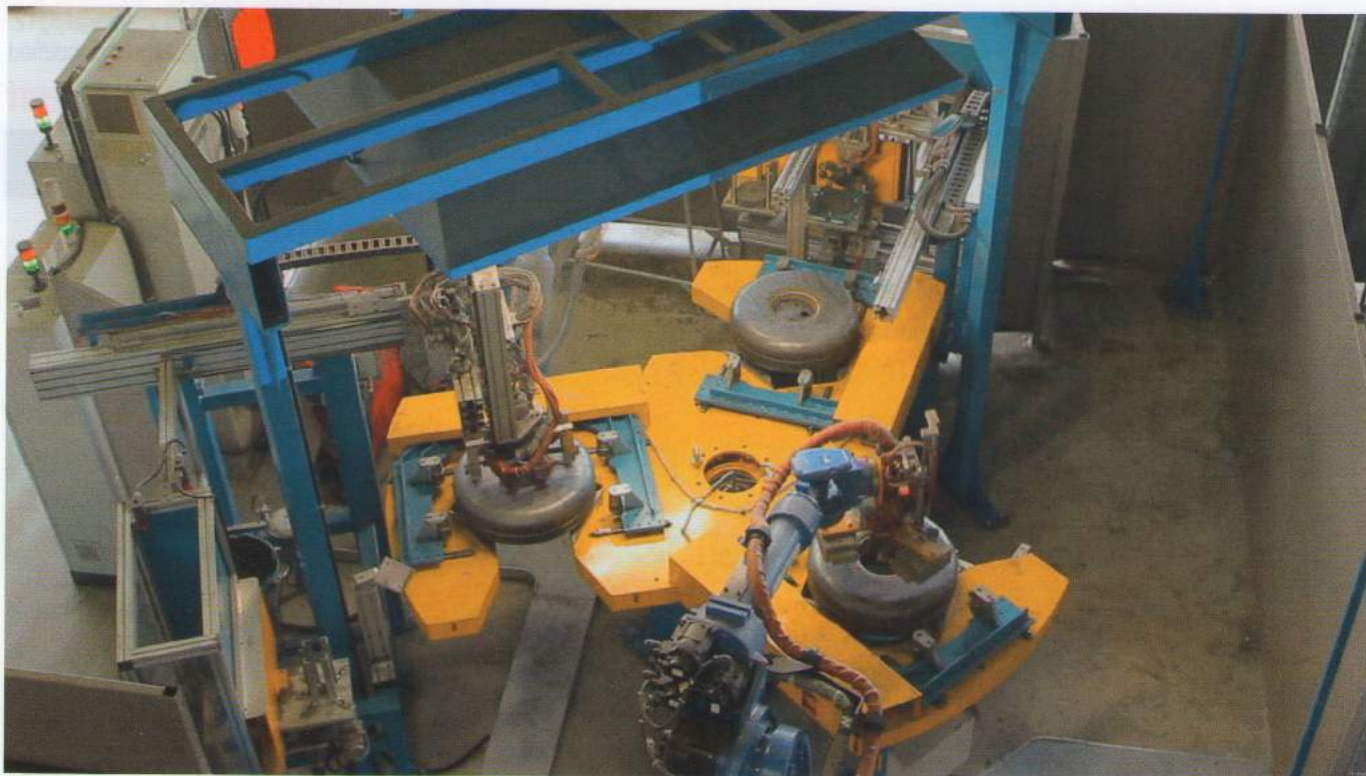
▲ Robotized toroidal tanks production line
