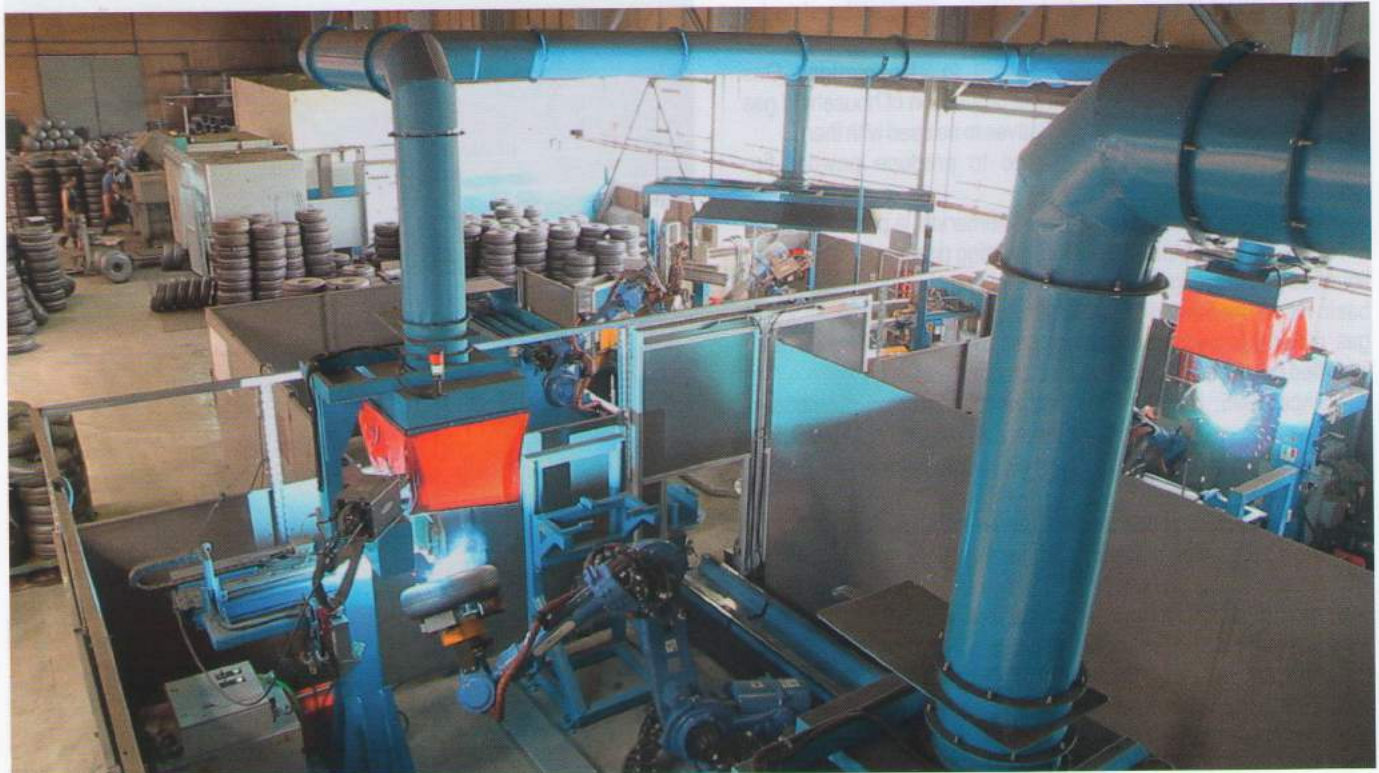
Robotized toroidal tanks production line ▼
