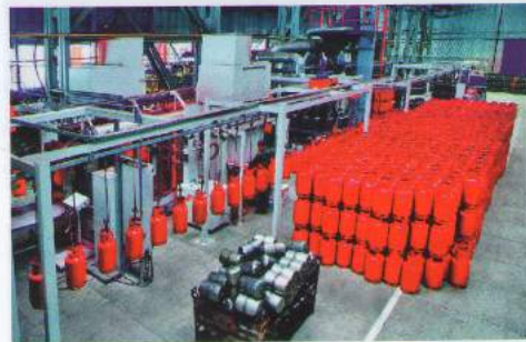
▲ Polymer painting line for gas European tanks
