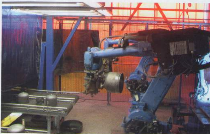
▲ Robotized welding line of cylinders 5l, 12 l and 27 l
